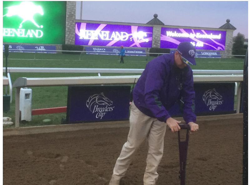
TIM FAHRENDORF, KEENELAND ASSISTANT TRACK SUPERINTENDENT, TAKING TRACK MOISTURE DATA USING TIME DOMAIN REFLECTOMETRY DURING THE 2015 BREEDER'S CUP RACES. PHOTO COURTESY DR. MICK PETERSON.
