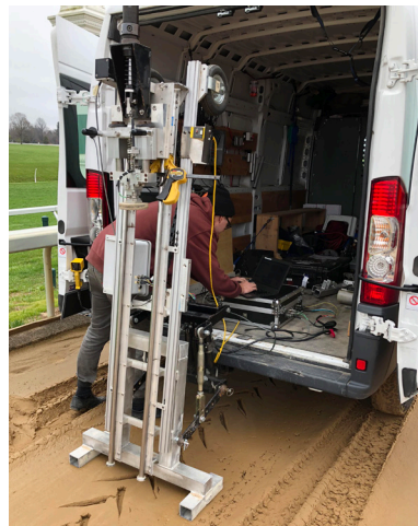
THE ORONO BIOMECHANICAL SURFACE TESTER (OBST) IS USED PRIOR TO EACH RACE MEET TO DUPLICATE THE LOADS AND SPEEDS OF THE FORELIMB AT A GALLOP. PHOTO COURTESY DR. MICK PETERSON.
