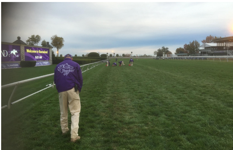
TIM FAHRENDORF, KEENELAND ASSISTANT TRACK SUPERINTENDENT, TAKING TRACK MOISTURE DATA USING TIME DOMAIN REFLECTOMETRY DURING THE 2015 BREEDER'S CUP RACES. PHOTO COURTESY DR. MICK PETERSON.
